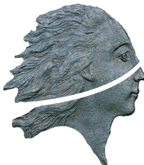
Figure 7. Illustration of the Chain cent hub showing the approximate location of the break, consistent with the overlays. The fine hairlines have been smoothed to show the waves more clearly.
