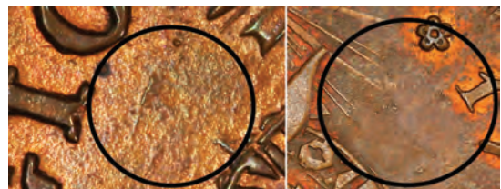
Figure 9. Left and right obverse field defects on later state brass strikes
